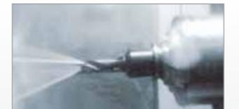
• Coolant Through Spindle
